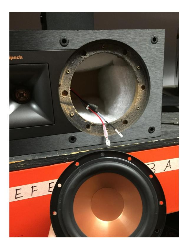
Next, plug the wires on to the new woofer, and slide the silicone covers back over the terminals.
