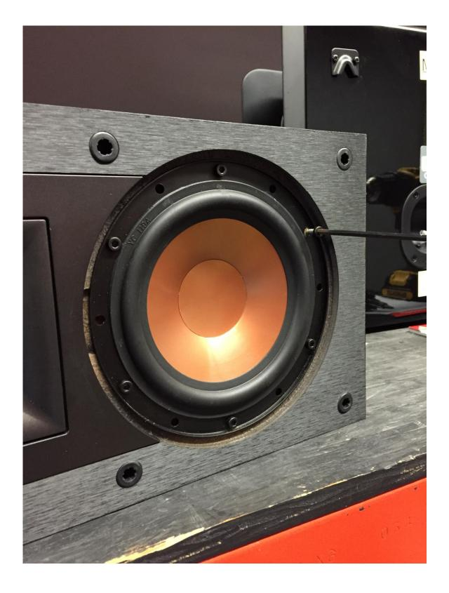
Once all the screws have been removed, the woofer should come free as shown below.
