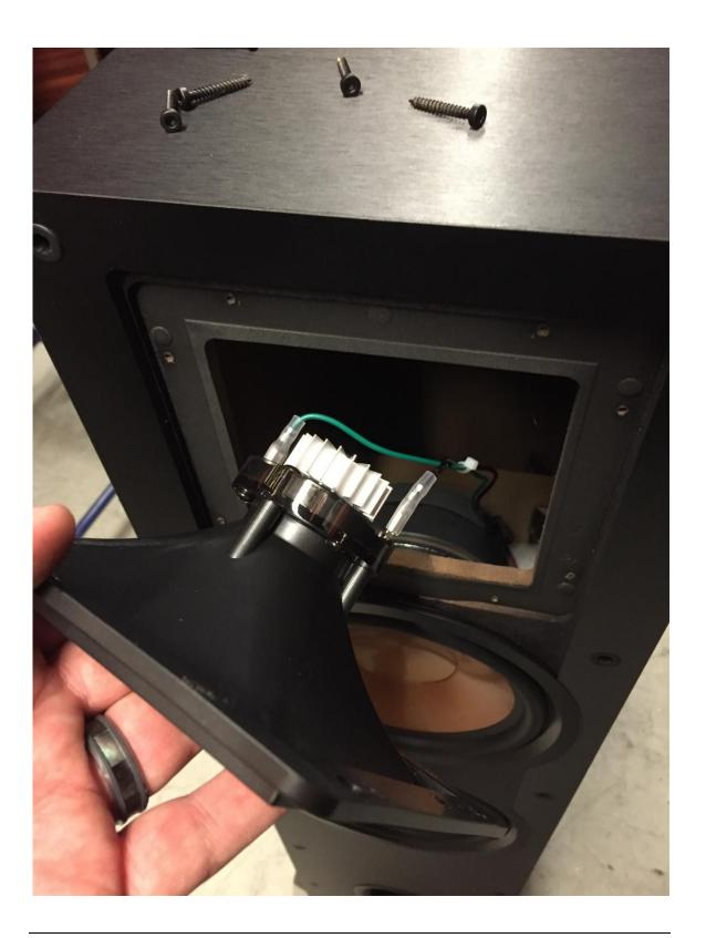
Once the tweeter is removed from the cabinet, slide back the silicone covers on the terminals, and use a small flat blade screw driver to release the wire clips holding to the positive and negative terminals of the tweeter.
