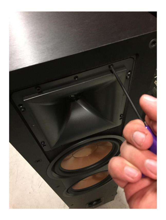
Once all the screws have been removed, the tweeter and tweeter horn should come free as shown below.
