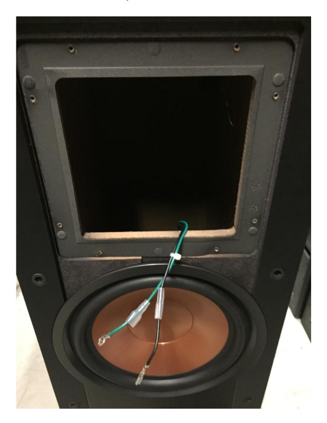
Next, plug the wires on to the new tweeter, and slide the silicone covers back over the terminals.
