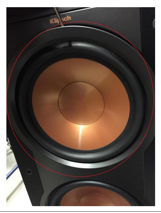
Be careful when removing trim ring around the edge of the cabinet, rough handling may cause damage to the cabinet
