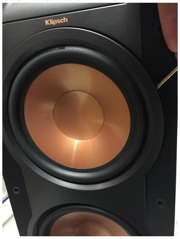
The trim ring comes off in a single assembly around both woofers as shown below.
