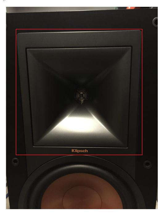
Be sure to pry the trim ring up in between the tweeter horn and the trim ring as shown below.
