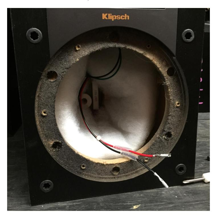
Next, plug the wires on to the new woofer, and slide the silicone covers back over the terminals.
