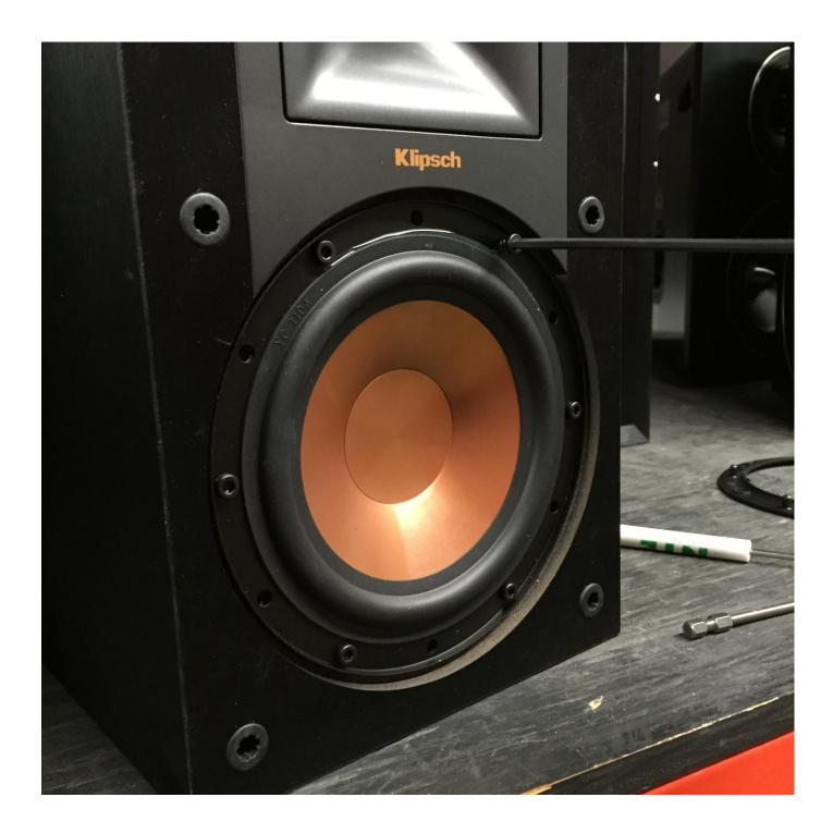
Once all the screws have been removed, the woofer should come free as shown below.
