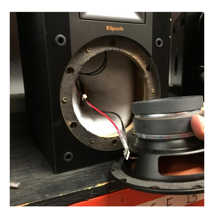
Once the woofer is removed from the cabinet, slide back the silicone covers on the terminals, and use a small flat blade screw driver to release the wire clips holding to the positive and negative terminals of the woofer.
