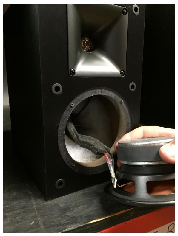
Once the woofer is removed from the cabinet, slide back the silicone covers on the terminals, and use a small flat blade screw driver to release the wire clips holding to the positive and negative terminals of the woofer.
