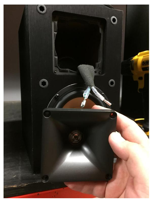
Next, plug the wires on to the new tweeter, and slide the silicone covers back over the terminals.
