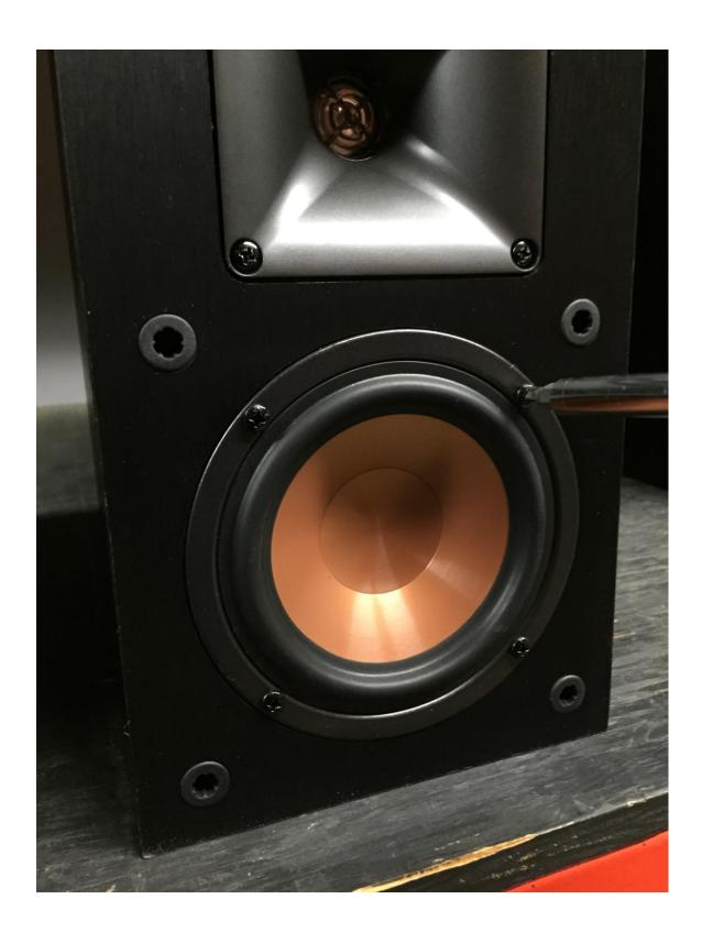
Once the screws are removed, the woofer should come free and appear similar to the picture below.
