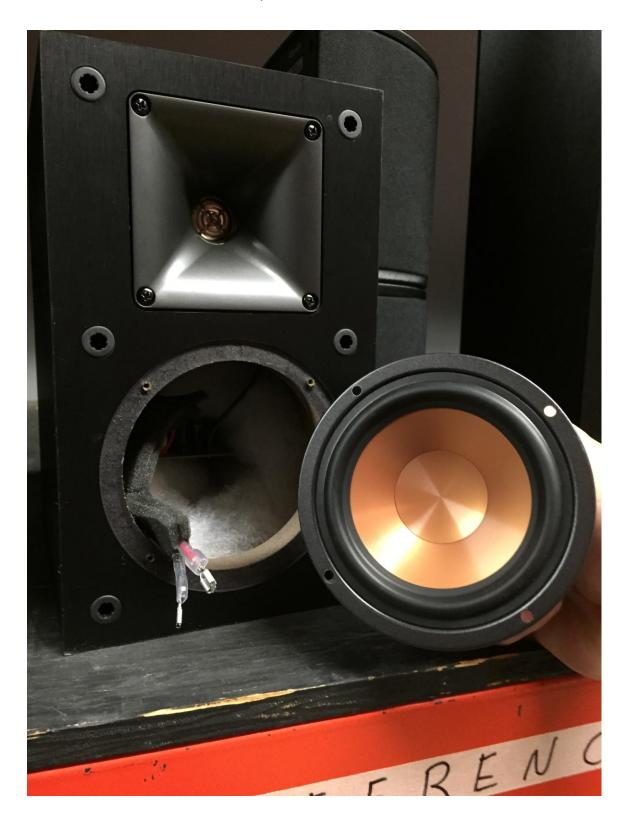
Next, plug the wires on to the new woofer, and slide the silicone covers back over the terminals.
